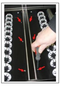
To reassemble and install the width array bank, reverse the procedure as described taking care not to pinch the cable as the width array assembly is screwed onto the platform.
