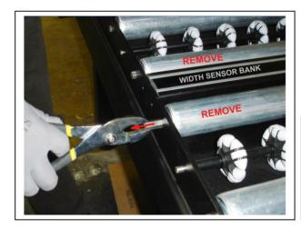
Use pliers to pull the conveyor roller axel toward the 480R front. As the axel retreats into the conveyor roller at the far end, lift the back of the roller up and then remove roller from platform.
