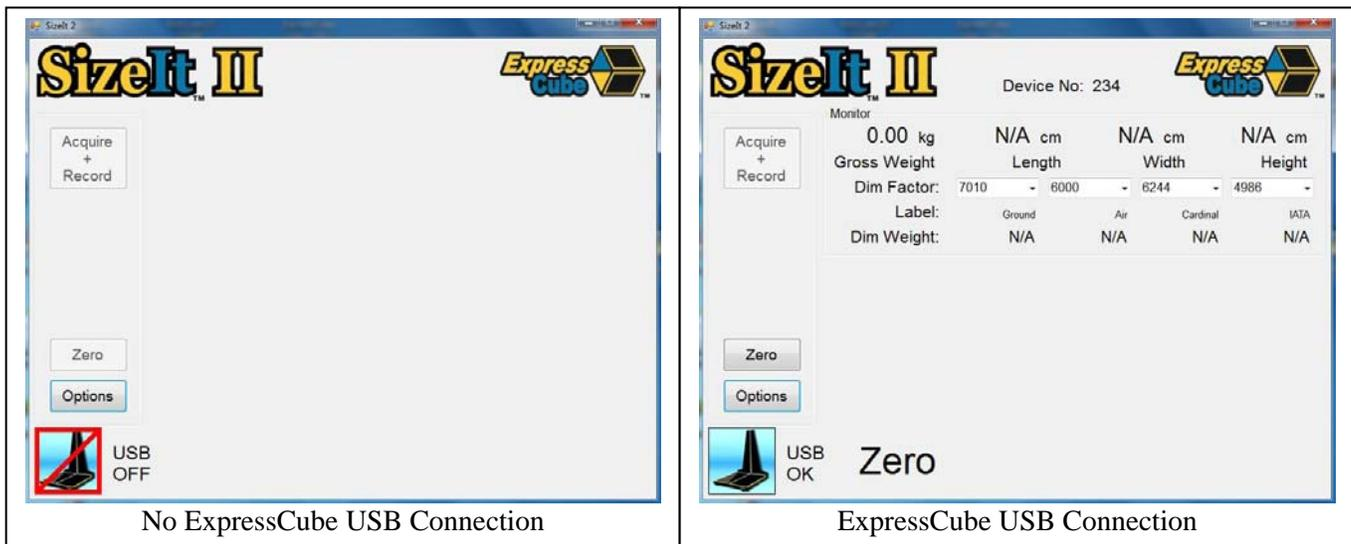
The SizeIt II screen should be as illustrated above. Press and release the ExpressCube platform to confirm the SizeIt II connection is made. If the USB connection is established, the platform weight will increase as you press the platform and decrease to zero (starting weight) as the platform returns to its resting position.
