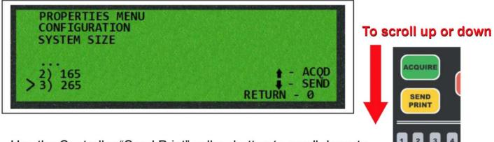
Use the Controller "Send Print" yellow button to scroll down to the desired size. The "Acquire" green button scrolls up. On the Cotroller, punch in the number next to the desired size to select a change.
