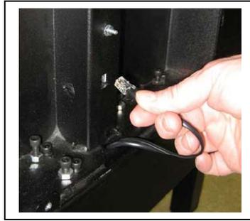
Install the longer cable into the LED Status board located at the top of the height assembly. >
