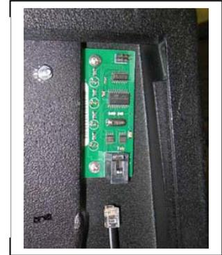
Slide the back cover into the slots and move the cover up to match up to the cover screw holes. Verify as the cover is placed that it is not pinching the cables in the height assembly. Secure the panel with the two small bolts as provided.
